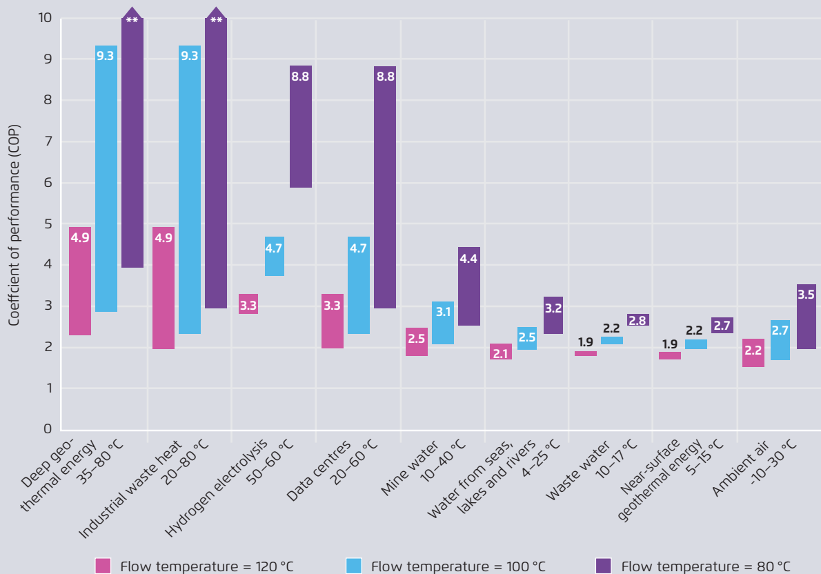
Theoretically possible COPs of heat pumps according to heat source and network flow temperature, assuming an efficiency rating* of 50% and different flow temperatures of the district heating network
